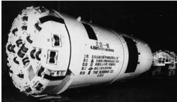
(a) Pilot TBM ( \phi=4.8 m)
