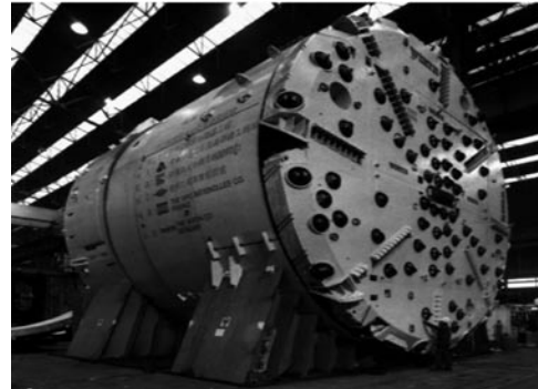
(b) EB and WB TBM ( \phi=11.74 m)
